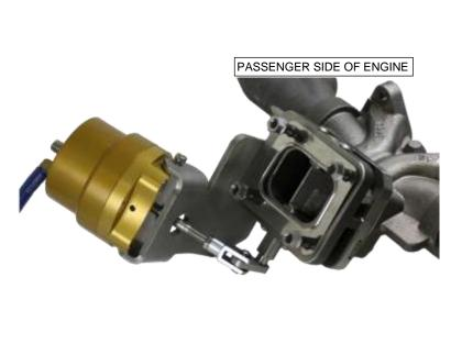
When the TDV is in the resting position it covers the front volute to direct exhaust gas to the lower part of the turbine wheel for better efficiency.
