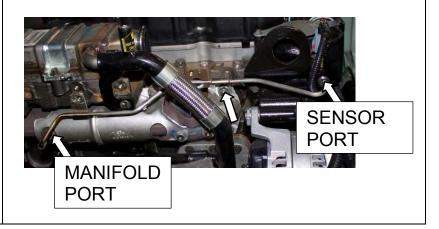
23. Remove two 15mm nuts securing EGR cooler to exhaust manifold at rear.
