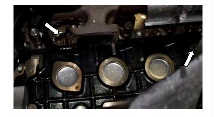
26. Pull coolant pipe out of the way and remove the locking tabs on exhaust manifold bolts.
