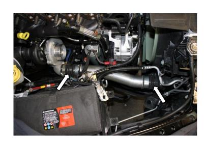
49. Remove coolant fitting from cylinder head with 1" wrench and install supplied pipe plug 3/8" square drive.
