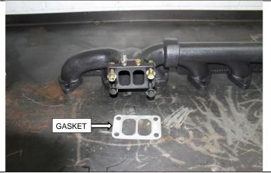
36. Attach turbo to BD manifold using the 2 supplied 3/8" NF X 1.5" bolts, nuts and washers inserted into the drilled holes and (1) M10 x 1.5 x 20mm bolt with flat washer in rear threaded hole. M10x1.5x30mm bolt and washer are used in the front threaded hole. (9/16"or 14mm wrench)
