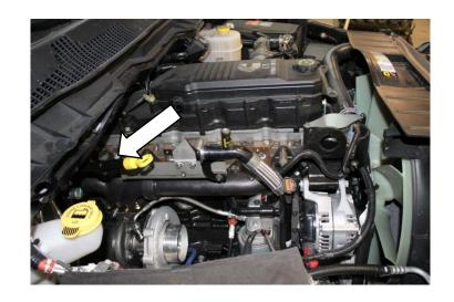
56. Remove and disconnect EGR valve from intake horn.4 (10mm bolts)
