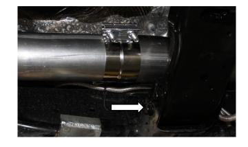
45. Preoil turbo by putting oil in through oil fitting then reattach oil feed line.
