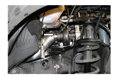
43. Reinstall exhaust hanger onto bell housing.
