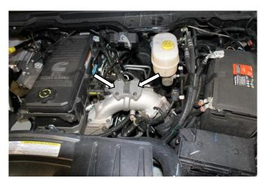
60. Reinstall air box and reconnect sensors. Then install the intake tube with PCV hose and secure PCV to bracket with OEM bolt.(10mm)
