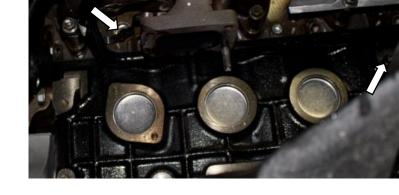
26. Pull coolant pipe out of the way and remove the locking tabs on exhaust manifold bolts.
