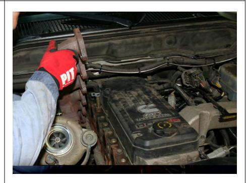
13. Remove the four nuts holding the turbo to the exhaust manifold with a 15 mm wrench. Then remove the two studs (double nuts each stud and turn out) from the factory manifold.
