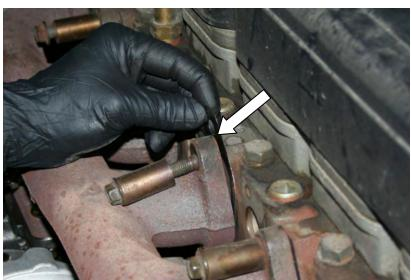
17. Reinstall the manifold heat shield.
