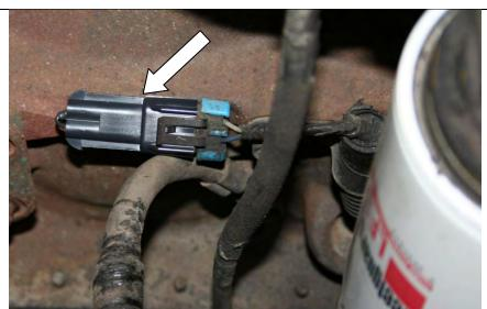
24. Install the intake hose then reconnect the air flow sensor.
