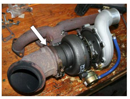
15. Before installing the Killer "B" turbo/manifold assembly clean the surface of the head that the manifold bolts to, and clean out any debris.
