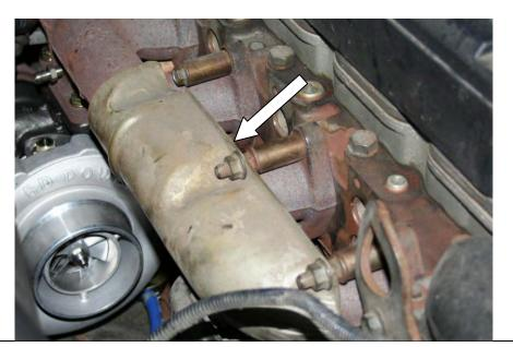
18. Reinstall the heater pipe bracket and tack weld back into position. It is suggest a small amount of black paint is used to paint the weld.
