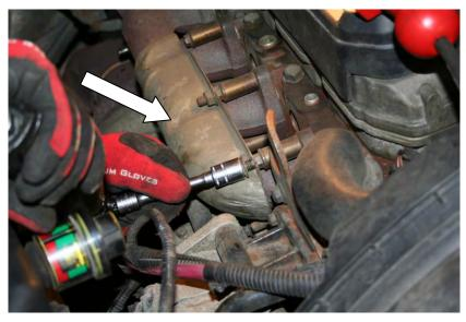
11. Then remove the rest of the manifold bolts using a13 mm deep socket.
