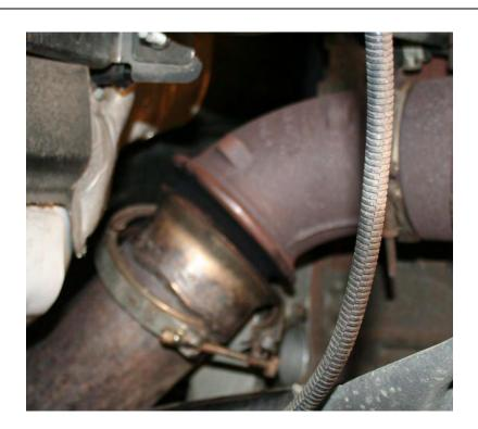
5. Remove the turbo oil drain line with a 10 mm socket.
