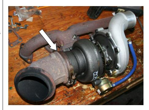
15. Before installing the Killer "B" turbo/manifold assembly clean the surface of the head that the manifold bolts to, and clean out any debris.
