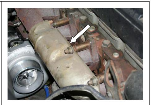
18. Reinstall the *heater pipe* bracket and tack weld back into position.
