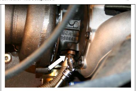
21. Secure the exhaust downpipe to cast adapter with the factory vband clamp.
