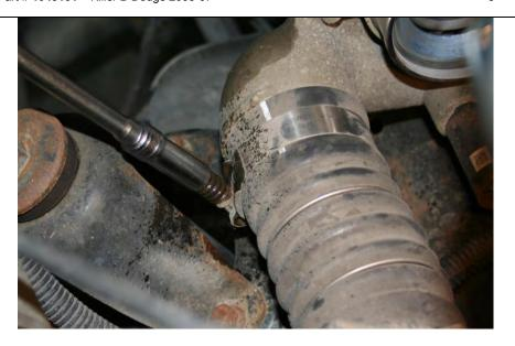
10. Pry off metal lock from rear manifold bolts, remove the heater pipe bracket from the manifold and remove the manifold heat shield with a 15 mm socket.
