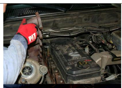
13. Remove the four nuts holding the turbo to the exhaust manifold with a 15 mm wrench. Then remove the two studs (double nuts each stud and turn out) from the factory manifold.
