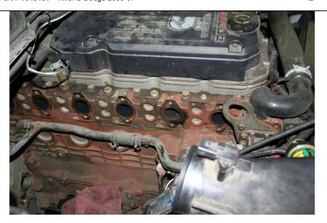
16. Carefully maneuver the BD turbo/manifold assembly back into the engine compartment and start two manifold bolts with the supplied gaskets.
