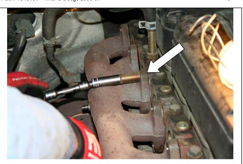
12. Remove the turbo/manifold assembly from the engine compartment.
