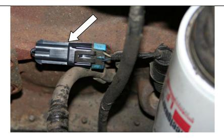
24. Install the intake hose then reconnect the air flow sensor.
