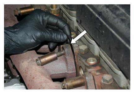
17. Reinstall the manifold heat shield.
