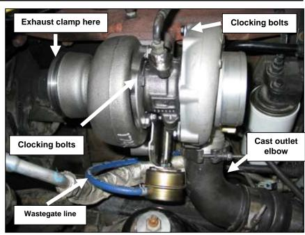
Ensure the orange o-ring is in place and use the factory v-band clamp to connect to compressor housing to the intercooler elbow and tube. Adjustment of the first intercooler boot may be required for a proper fit.
