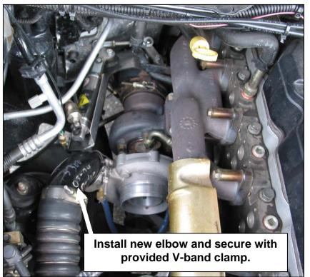
the Install powder coated compressor outlet elbow, o-ring, and V-band clamp. At this time you may insert the intercooler tube that you removed earlier. Don't forget to clean and secure all intercooler boots and tighten the hose clamps. When re-installing the intercooler tube, rotate the tube so that it is clear and free from either the air box or the plastic inlet tube. As well be careful that the compressor outlet elbow does not contact the shock tower.
