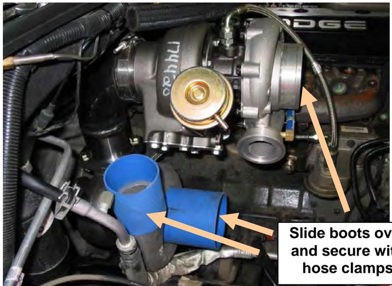
48. Install a 4 inch silicone boot on both the *primary turbo* and *secondary turbo* compressor housing inlets – also slide two Heavy Duty 4" band clamps on to each boot for easier installation later.
