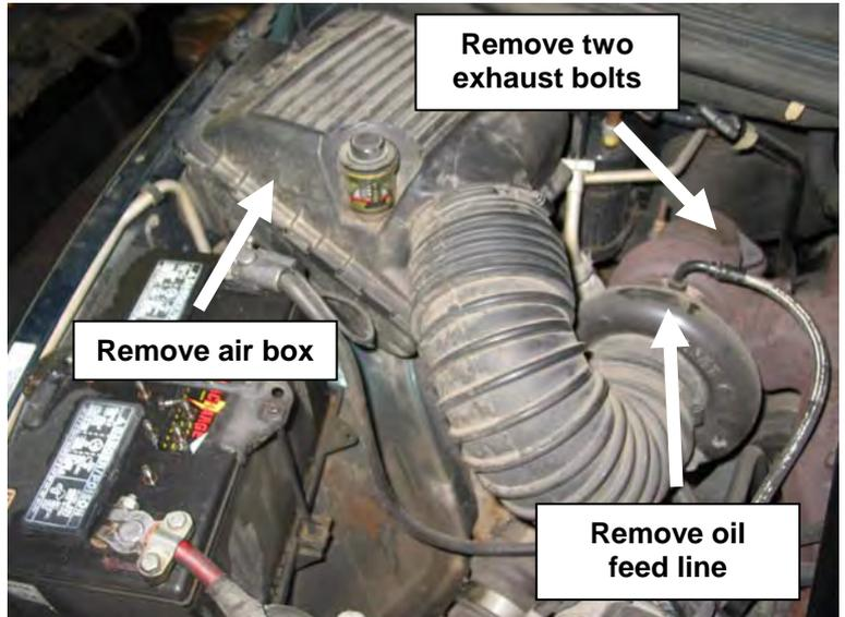
6. Remove the black steel intercooler tube. You will need to loosen the band clamp on the intercooler using a 7/16" deep socket.
