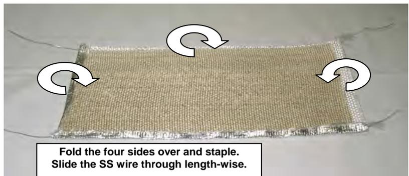
55. Install the turbo heat shield as shown over the top of the secondary turbo exhaust housing and secure with the stainless wire. Completely wrap the blanket around the turbo housing, then tighten and tie off with the stainless steel wire.
