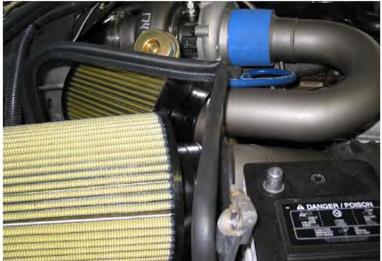
**Note:** The exhaust housings of the turbos may smoke slightly when new, as manufacturing residue on housing must burn off.
