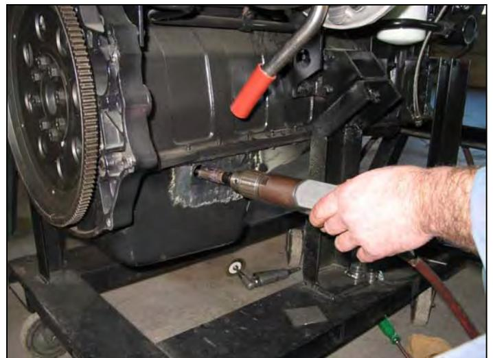
31. Center punch the pan 1 3/16" from top lip between the 3<sup>rd</sup> and 4<sup>th</sup> bolts
