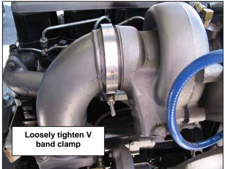
30. Install the *primary turbo* support bracket to the engine block with the supplied bolt (12mm x 1.75 x 25) and lock washer. Now tighten the bolts and V band clamp.
