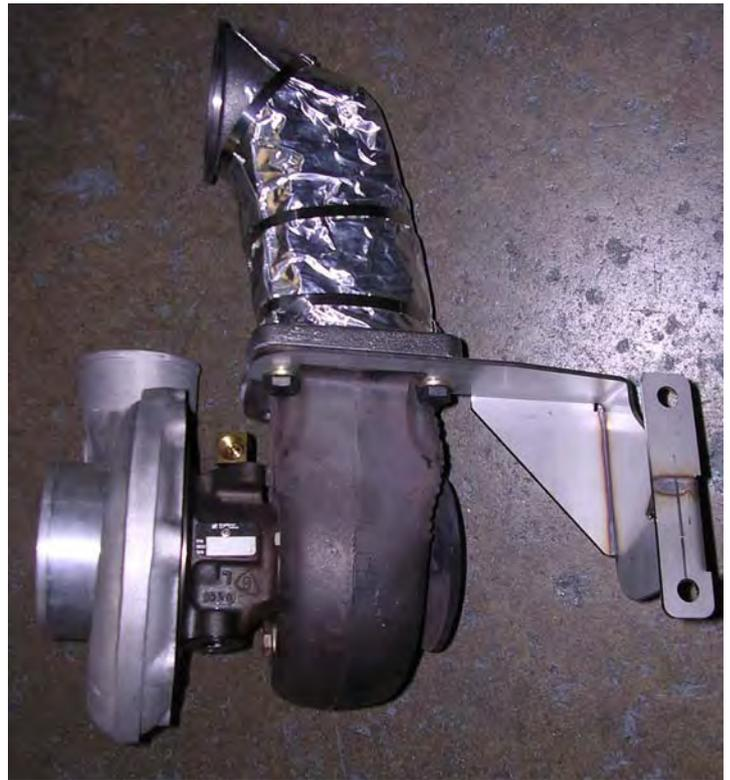
27. Place the turbo and turbine adapter assembly onto the frame rail in a location close to the final install point. Be sure that it does not fall.
