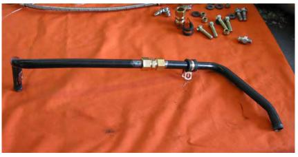
manifold and hook it back up to the factory rubber hoses. Once positioned, tighten the brass coupler and install the new support clamp to the oil filter housing bolt. Zap strap the two rubber heater hoses to secure them together.
