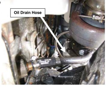
attach to the factory drain adapter. Use the hose clamps to secure the connection. You will need to slide the oil drain adapter as far as possible away from the wastegate arm to prevent any contact. In some rare cases the wastegate arm may need to be bent.
