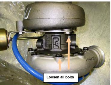
the turbo wheels. The clamps should only be loose enough to clock the housings.
