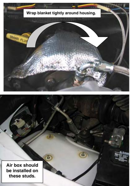
compressor-housing inlet of the *primary turbo*. Install air box onto the factory BD ENGINE BRAKE, INC. studs using the three supplied  $\frac{1}{4}$ " NF nuts and the three supplied  $\frac{1}{4}$ " flat washers.
