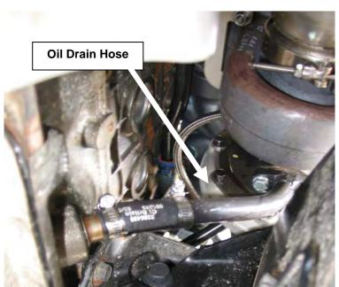
feed adapter in the *primary turbo*, making sure that it points towards the engine with the compressor housing facing forward.
