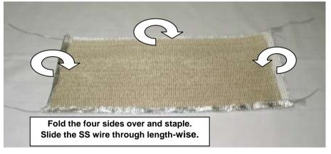
Note that the silver side should be facing out, so that the tan wrap is fixed against the white side of the wrap. You will need to staple all four folds to secure them in place. Once secure, run the 40" stainless wire through the folds
