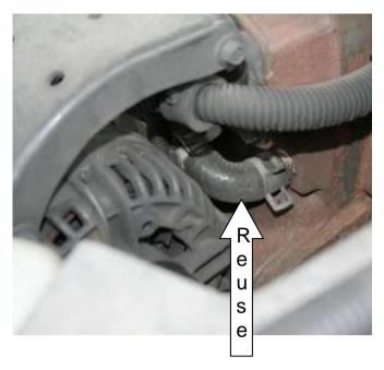
24. Also remove the coolant line at the side of the aluminum distribution block beside the lower radiator hose.
