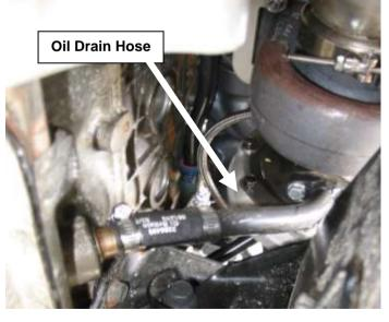
need to slide the oil drain adapter as far as possible away from the wastegate
