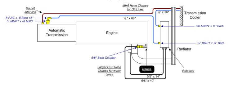
Using the 90° formed rubber hose that you saved earlier, install it on the passenger side front of the engine cylinder head. Secure the connection using a HS8 clamp. On the other side of the rubber 90° insert the 5/8 barb coupling (1452820). Secure the connection with another HS8 clamp.
