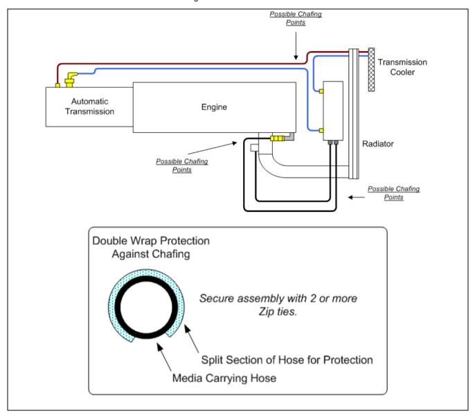
You can now start on routing the transmission oil lines. First connect the  $\frac{1}{4}$  MNPT x -8 MJIC (1604048M) fitting to the transmission cooler port ont eh driver's side of the transmission. Use a small amount of pipe sealant on this application, thread the fitting in by hand and then using a wrench give it one more turn and no more. **Do not over torque.**
