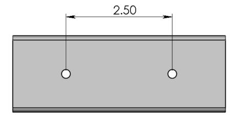
31. Then secure the two mounting brackets (1453118) to the cross member using the 7/16" mounting hardware(1452816, 1452817, 1452818, 1452819). Torque the bolts to 20 ftlbs. Note that the "windows" or rectangular clamp cutouts should be vertical.
