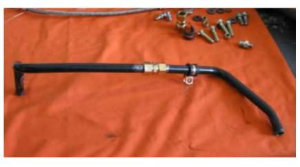
end between the turbo and manifold and hook it back up to the factory rubber hoses. Once positioned, tighten the brass coupler and install the new support clamp to the oil filter housing bolt. Zap strap the two rubber heater hoses to secure them together.
