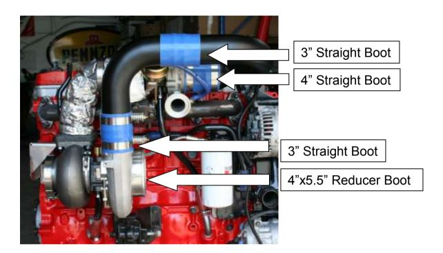
Install one 4" silicone boot on the secondary turbo compressor housing 60. inlet. Slide two heavy duty 4" spring band clamps (4.11) at the same time, you will need to completely loosen the nuts to do this.
