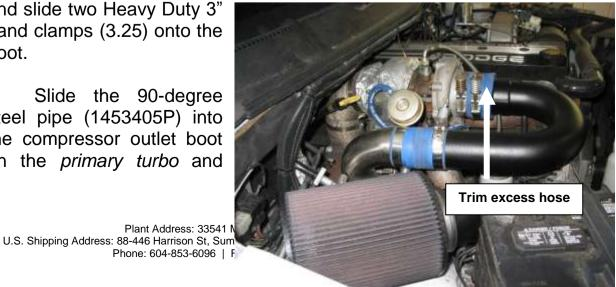
point the pipe outlet towards the front of the vehicle.
