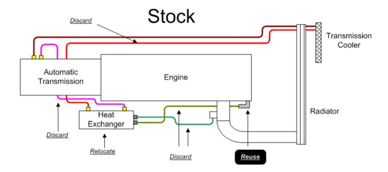
23. Then disconnect the coolant line at the front passenger's side of the engine from the 90° rubber bend/elbow. Just loosen the hose clamp to release the hard line. Note that you will need to keep this 90° rubber bend/elbow in place.
