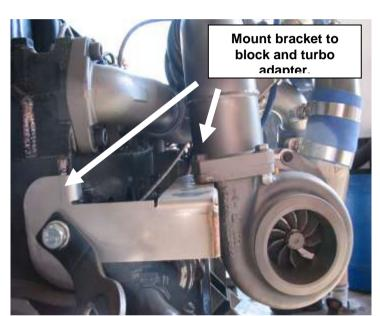
adjust the factory block oil drain adapter to help align the system.
