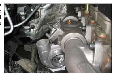
47. With the secondary turbo, bolt it loosely to the manifold and align the oil inlet straight up and the compressor outlet towards the bottom of the passenger battery.
