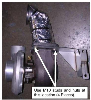
46. Place the turbo and turbine adapter assembly onto the frame rail in a location close to the final install point. Be sure that it does not fall.
