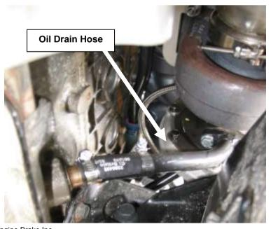
40. Install the short oil drain adapter onto the bottom of the r700 *primary turbo* with the supplied gasket and two M10x1.5x25 bolts and M10 lock washers.
