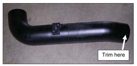
before re-installation into the 4"-5.5" silicone boot. Use the previous 4" gear clamp to secure the boot onto the inlet tune. Reconnect the filter and Air Mass sensor.
