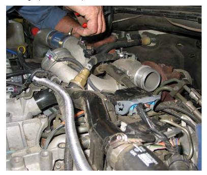
Using a 10mm socket, remove the air intake heater connection, MAP sensor mounting bolt, and unplug the MAP sensor.
