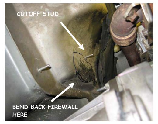
Using a larger pry bar, massage the firewall in the area shown, being careful not to pry against anything that will break. There is an engine-lifting bracket on the back of the passenger side head that works well as a leverage point. This is necessary to accommodate the larger down pipe.
