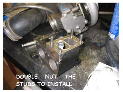
Install the two step studs for the oil drain spacer into the bottom of the turbo and tighten with vice grips. Install the oil drain spacer with a gasket on each side.
