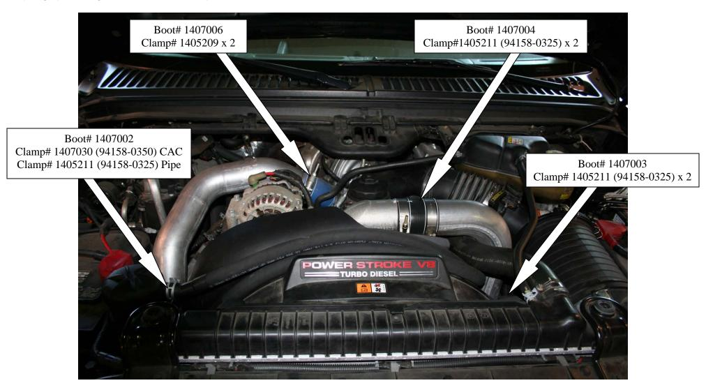
Place clamp over top of internal ribbed section.
