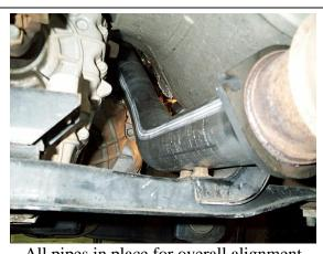
All pipes in place for overall alignment
