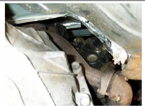
With the OEM pipe removed, ensure the firewall is flattened to provide clearance for the new pipe.
