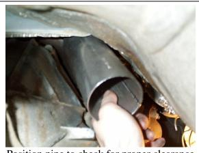
Position pipe to check for proper clearance
