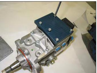
Screw in the retaining screws until they are snug. **Do not over-tighten them**.
