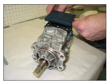
Place the plastic cover supplied in the kit on top of the pump, with the flat side up and lining up the holes for the 5 retaining screws.
