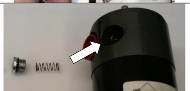
When reinstalling the plug and spring assembly, ensure the spring is centered in the piston.
