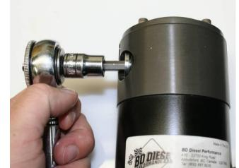
Once the plug is removed you can access the spring to be changed.
