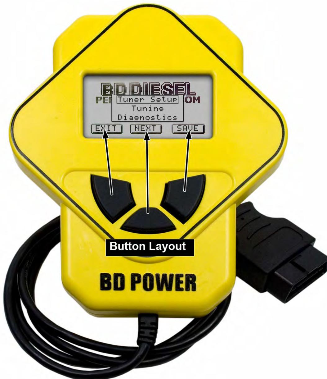
The layout of the BD Ultra X-Power tuner is pretty straightforward. The module consists of a graphical LCD display, 3 selection buttons (notice the relation to the placement on the screen) and an OBD-II communications cable, hardwired into the module.
