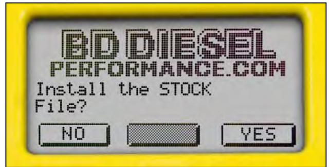
When the load is finished, the Ultra X-Tuner will have returned the vehicle to the stock power level, as well as the speed limiter and the transmission shift patterns.
