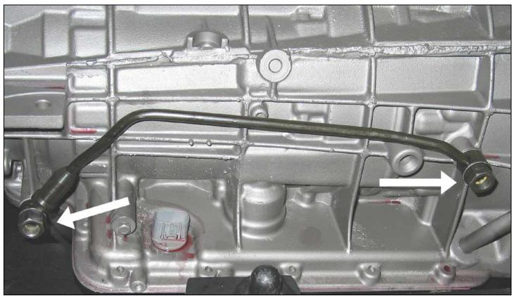
Remove the transmission cooler bypass hose by removing the two (2) Banjo bolts.
