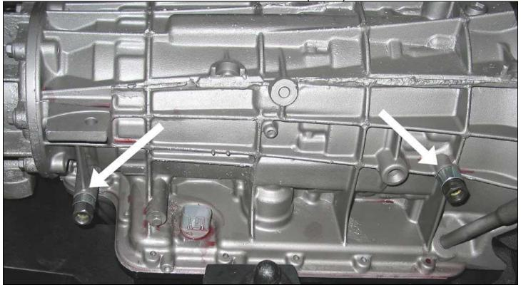
Install by-pass flanges in place of by-pass tube with new Banjo washers.
