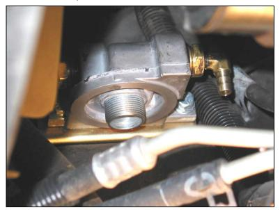
Position the filter head on the filter mount and secure using the 3 mounting bolts and washers supplied. Leave the filter off at this point as it will be installed later.
