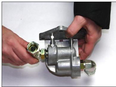
Install the two **90° ORB fittings** into the filter head (do not use pipe sealant). When installed, the fittings need to point in a downwards direction, towards the filter. For ease of installation, we recommend assembling the fittings on the filter head on a work bench before installing it onto the vehicle.
