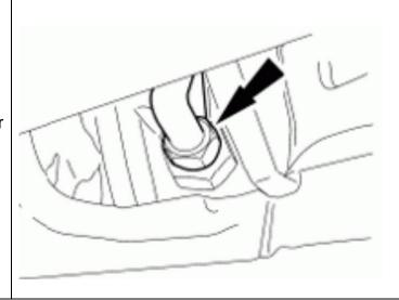
14. While holding the case fitting, remove the front transmission cooler tube.
