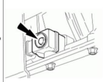
10. Disconnect the output shaft speed (OSS) sensor.
