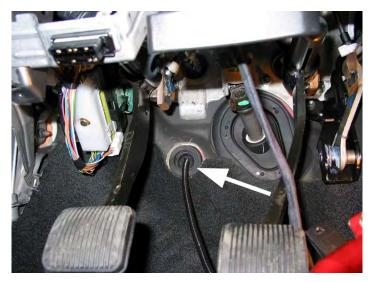
Open the loom and locate the Light Blue w/Black wire and install a gray Posi-Tap<sup>TM</sup> to it.
