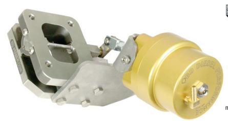
Variable Turbocharger Geometry control with BD's Turbine Diverter Valve improves turbocharger response at low engine rpm by feeding all the exhaust gas flow through one
