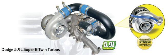
BD's Super B Twin kit features a pair of stage-compounded AirWerks \$300 turbochargers to keep air flow high and exhaust gas temperature (EGT) low. The high-pressure turbo provides quick, low-rpm response, which compounds the low-pressure turbo for a broad power curve across the engine's rpm range.
