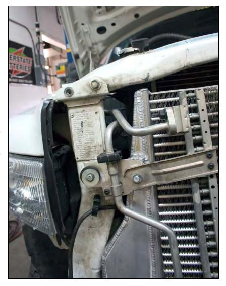
You will need to re-use the two factory rubber spacers to secure the new intercooler.
