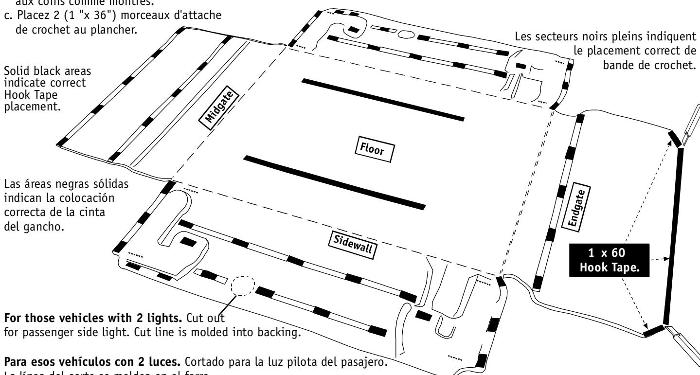
**3** Lay midgate down and lay BedRug in vehicle. Align for best fit by using cargo hook and cargo light openings for reference.
