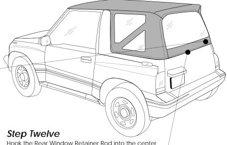
Hook the Rear Window Retainer Rod into the center bracket on the tailgate and then into the bracket on each side of the tailgate.
