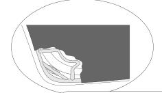
Note: To close Side Panel Retainer, push the retainer into the clip mounted to the body.
