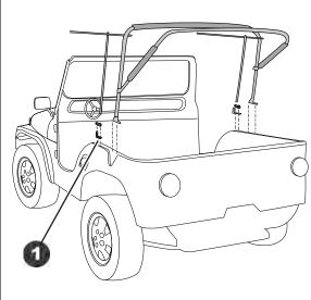
CJ5 Windshield Adjustment: If necessary, loosen the two screws in the Windshield Clamps at the base of the windshield on each side of the vehicle. Adjust the windshield forward or back, use a shim if needed to position the windshield, and tighten the screws.
