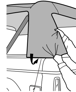
Slip Plastic Retainer into Channel in Side Belt Rail
