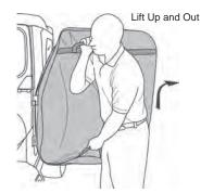
If removing Lower Steel Door with Soft Upper, always lift the door from the bottom, grasping the steel door section.
