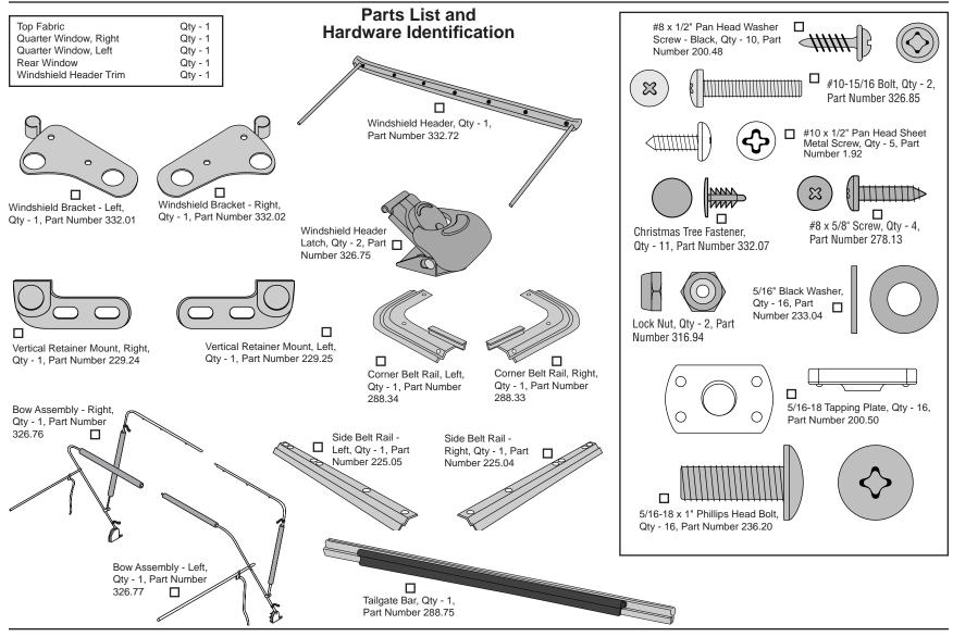
**NOTE** If you are replacing an old soft top, be certain that all parts of the old top are removed, including the windshield retainer. Old metal parts are not compatible with the new Supertop. Using parts other than those provided in your Supertop kit can result in personal injury and/or damage to the vehicle and soft top.
