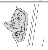
Special Note: The Rotary Latch Paddle Handlevill only latch on the automobile manufacturer's original equipment steel latch pin located on the vehicleDo Not adjust or remove this part.
