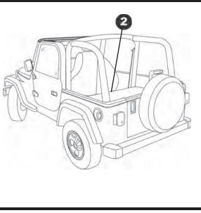
Check for wiring and fuel WARNING lines before drilling holes in riser.
