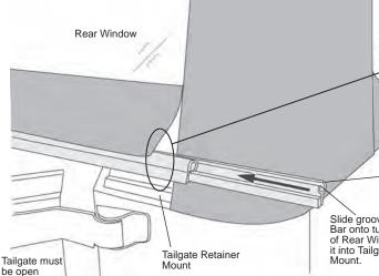
Rear Corner Retainer Tailgate Bar Slide groove in Tailgate Bar onto tube on inside of Rear Window. Push it into Tailgate Retainer
