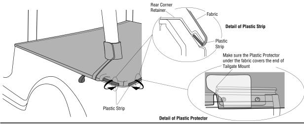
Note: The Plastic Protector sewn into the fabric must be located over the Tailgate Retainer Mounts.
