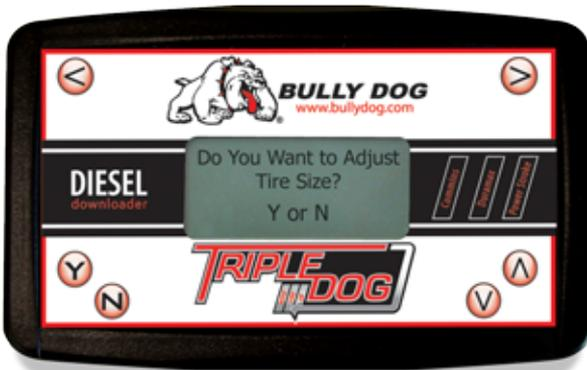
**WARNING:** Adjusting above 35" for tire size many cause the ABS lights to come on.
