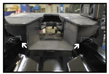
Reinstall the hitch head assembly. Mark and trim the head to allow the proper 10-1/2 degree downward tilt. Reinstall the hitch head pins.
