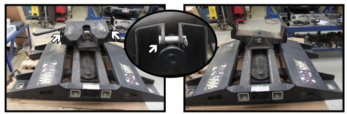
1. Remove the pins, one (1) on each side, from the hitch head assembly and remove the hitch head assembly from the base.
