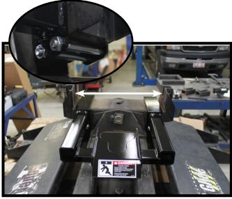
Install the Bedsaver<sup>™</sup> onto the hitch and center on the base. Use 1/2"-13 x 7-1/2" bolts and 1/2" lock nuts to fasten to the base.
