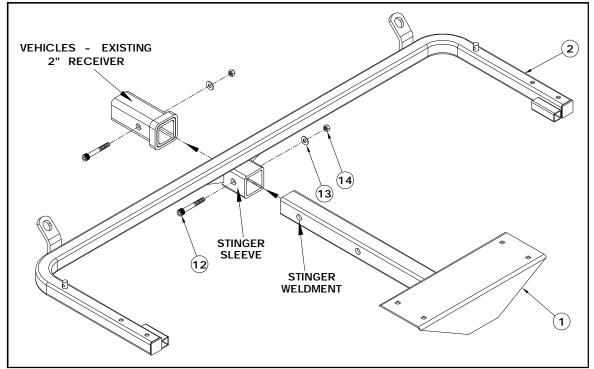
Insert stinger weldment into the stinger sleeve and tow vehicle's receiver to align 5/8" pin holes. Insert 7/16-14 x 2 3/4" cap screw (item 12) into receiver, tighten flat washer and 7/ 16-14 hex nut using the 11/16" socket and 3/8" allen wrench. Torque 7/16-14 hex nuts to 54 ft. Ibs. Slide stinger sleeve back, align holes of stinger and sleeve. Insert 7/16-14 x 2 3/4" cap screw into hole, put on the 7/16" flat washer and 7/16 nylon hex locking nut. But do not tighten.
