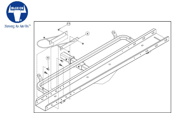
3. Slide the tire support weldment flats (item 4) on the outside edge of the narrow end on the motorcycle deck (item 3) to align the square holes of the deck with the round holes on the tire support. Insert the 3/8-16 x 1" carriage bolt into the square holes on the inside track of decking and tire support, tighten the 3/8-16 nylon hex locking nuts on the outside edge of tire support flats with the 9/16" socket. Torque 3/8-16 hex nuts to 33 ft. lbs.
