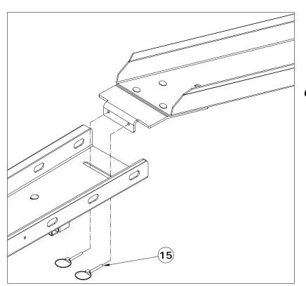
6. To prepare your motorcycle carrier for loading, remove the ramp from the motorcycle carrier, set the connecting plate flange into the slot at the end of the deck and insert the quick clips into the holes in the flange to stabilize the ramp for loading.
