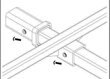
**NOTE:** The head of the 7/16-14 x 2 3/4" cap head screws are recessed into the 5/8" opening of receiver and stinger sleeve. This will allow stinger to be pulled to one side and eliminate stinger to wobble.
