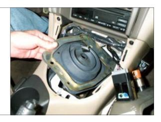
STEP 8. Remove four (4) shifter base bolts.
