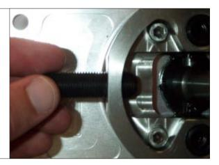
STEP 11. Thread jam nuts onto shift stops.
