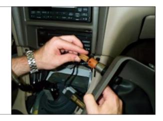
STEP 4. Remove four (4) bolts from protective boot.
