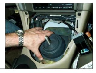
STEP 21. Install four (4) bolts securing protective boot.
