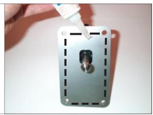
STEP 17. Install B&M Pro Ripper Shifter. Part: B&M Pro Ripper Shifter
