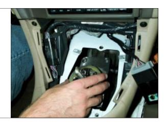
STEP 18. Install four (4) washers and four (4) mounting nuts.
