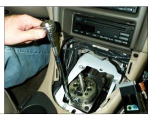
STEP 19. Adjust shift stops accordingly.
