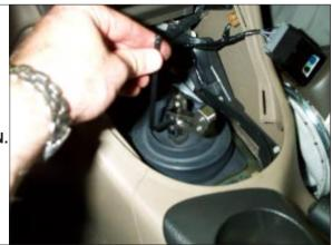
STEP 25. Install threaded knob adapter.
