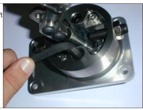
STEP 15. Install four (4) mounting studs. Tools: 4mm Allen wrench Parts: Mounting studs
