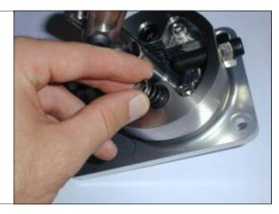
STEP 14. Reinstall socket locks in shift stop ring.
