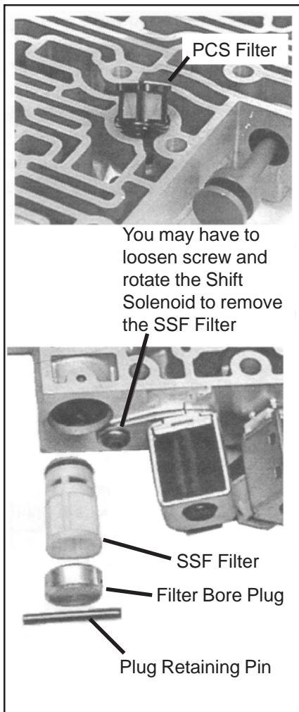
Figure 4: PCS and SSF Filters
