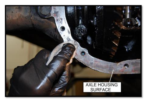
clean the accessible areas of the axle housing and check internal components for visible excessive wear or other problems.
