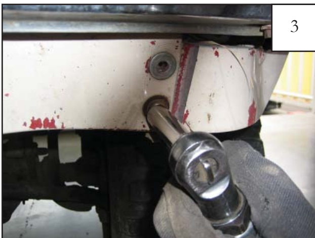
3 Using a 10mm socket, remove two factory fasteners underneath bumper on either side. Remove fascia piece.
