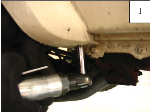
1 Remove the front factory flare starting with the lower rear factory fastener, using a 7mm socket.
