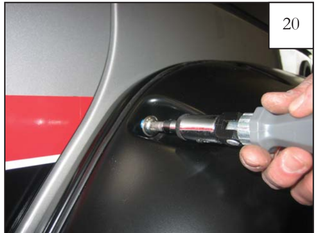
Start Screws/Washers through pocket holes in flare and into Threaded Clips installed in Step 11 (8 places) starting at the front and working your way to the back. Do not tighten.
