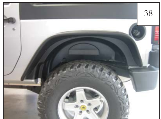
Completed rear driver's side flare installation.
