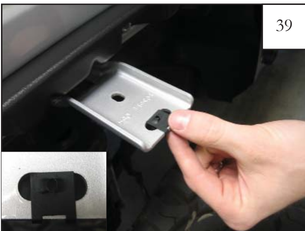
Before installing the outer flare, install speed clip on metal frame angle support bracket at top center of wheel well. Make sure that it is centered over the factory slot with threaded portion facing up.
