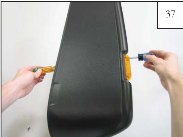
Secure the side marker light to the outer flare with 8-32 screw, 8-32 nut, and washer using a #2 Phillips bit and a 11/32" socket with 8" extension (2 places). NOTE: If you are having trouble putting the washer and nut on the screw, use needle nose pliers.
