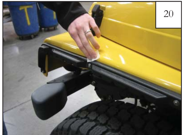
20 Use one supplied alcohol prep pad to clean the sheet metal above each inner piece in preparation to tape the edge trim to the sheet metal. This must be done for proper flare installation.
