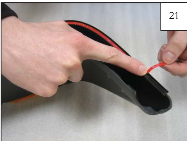
21 Peel back 1-2" of red liner on each end of the edge trim and bend toward the outside of the flare.
