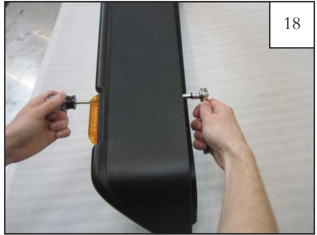
18 Secure the side marker light to the outer flare with 8-32 screw, 8-32 nut, and washer using a #2 Phillips bit and a 11/32" socket with 6" extension. (2 places) NOTE: If you are having trouble putting the washer and nut on the screw, use needle nose pliers.
