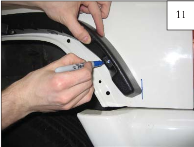
Align outer edge of inner piece P1 (D1 for driver side) with the measuring line made in Step 9. Use a grease pencil or marker to mark the front hole location on the sheet metal.
