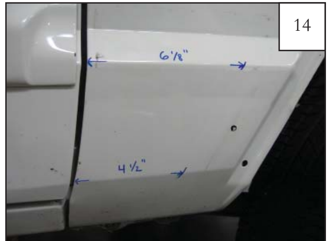
Use a grease pencil or removable marker to mark a line parallel to wheel well opening 6-1/8" from the door edge seam along style line and 4-1/2" on lower style line.
