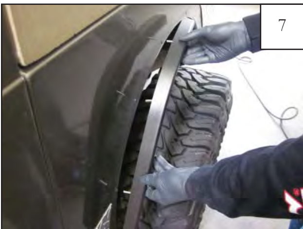
Secure inner piece D3 (and P3 for passenger side installation) to the sheet metal using the following 3 STEPS: Step 1 Line up the Screws (SW1-0053) with the factory hole locations.
