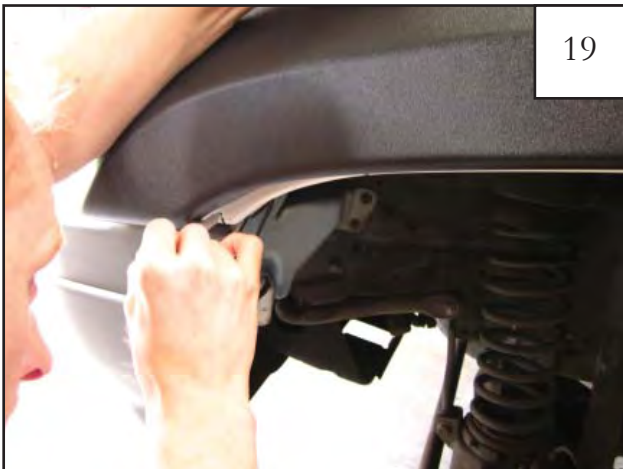
Hold the flare up to the fender as a guide. Make a mark connecting the two marks made in step 18.
