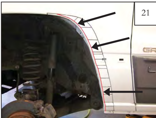
Make a mark approximately 1/4 " in from the edge of the wheel well lip starting at the bottom of the wheel well extending to the uppermost point of the markings.
