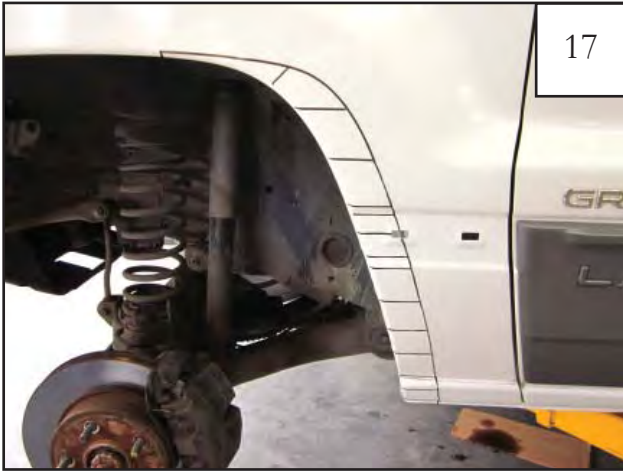
Mark vehicle for cutting: Make horizontal marks from wheel well to line drawn in previous steps about two inches apart as shown in picture. Make marks closer together around tight corners and style lines.
