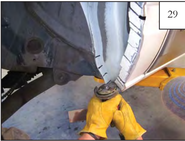
Using a cutoff wheel or other suitable tool, starting at the bottom line, cut horizontal marks in the pinch weld.
