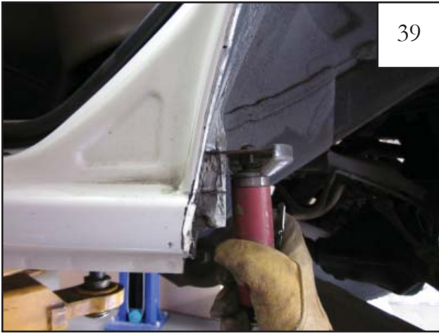
Using a cut off wheel or other suitable tool, cut along horizontal marks made in step 37.
