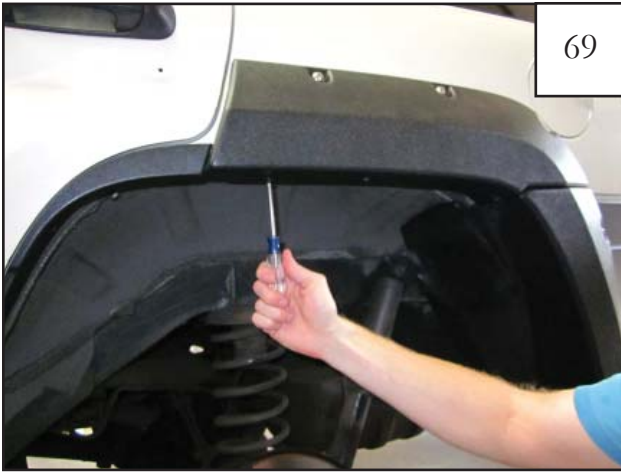
Secure flare to fender with panhead screw (SW1-0056) through holes drilled in step 68.
