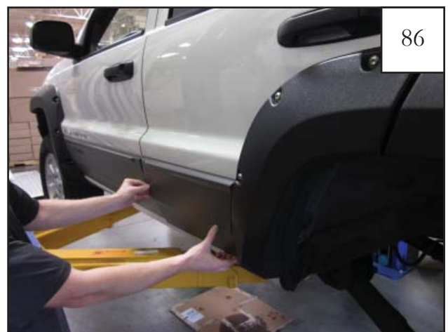
Hold cladding in place on vehicle and re-attach by pressing firmly along upper edge to fasten into factory hole locations on sheet metal.
