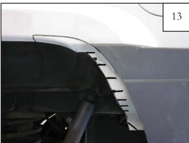
Mark vehicle for cutting: Make lines on sheet metal as shown in picture.
