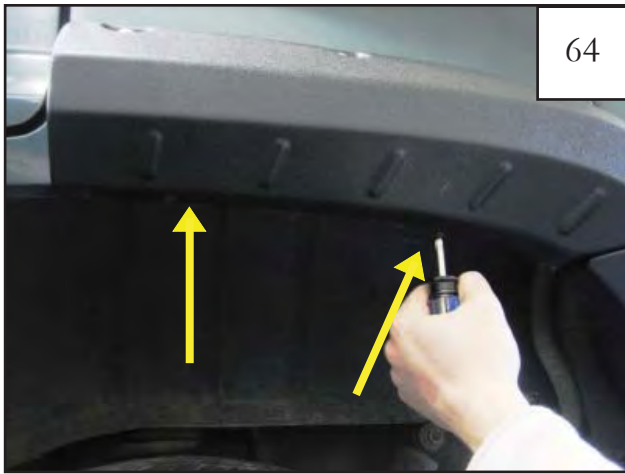
Secure flare to fender with the #8 pan head screws through holes in flare and into predrilled holes. A drill with a #2 Phillips driver works well.
