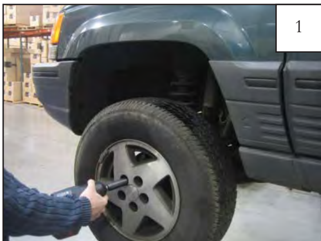
Remove tire using an impact wrench.
