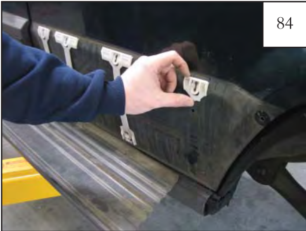
Reinstall top portion of side cladding clip on vehicle.
