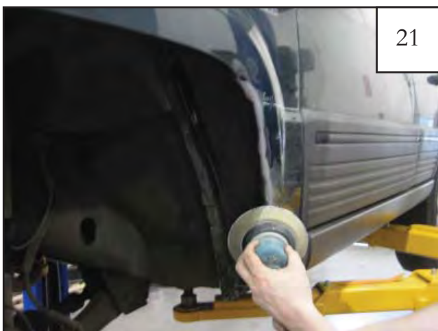
Sand the chipped paint along bent edge of the wheel well.
