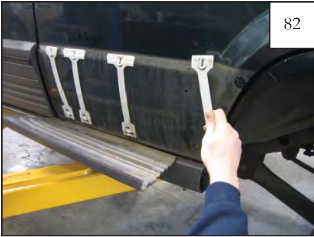
Remove cladding clip closest to the rear wheel well.
