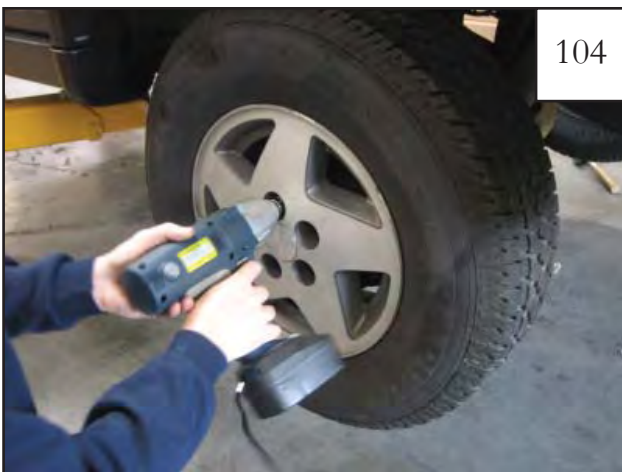
Reinstall the tire using an impact wrench.
