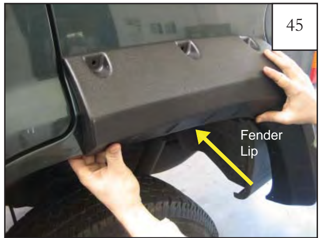
Hold the assembled flare in place on vehicle aligning forward edge with door seam and inside of rear main part with fender lip. NOTE: See step 46 about gapping between bumper and bumper piece.
