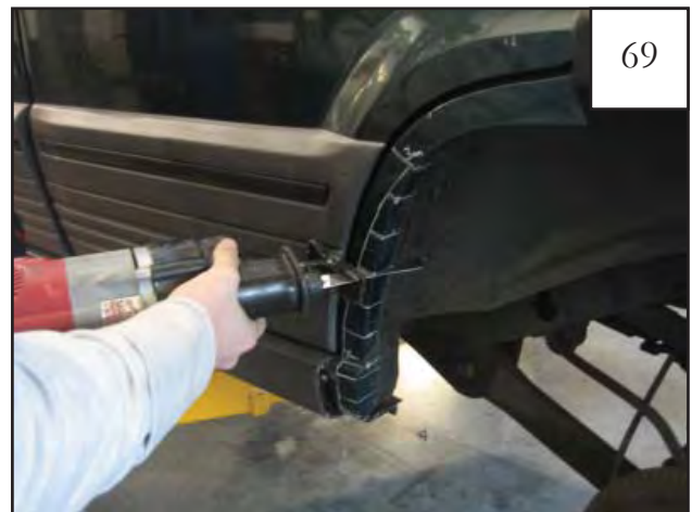
Cut horizontal marks from wheel well to vertical line with reciprocating saw.
