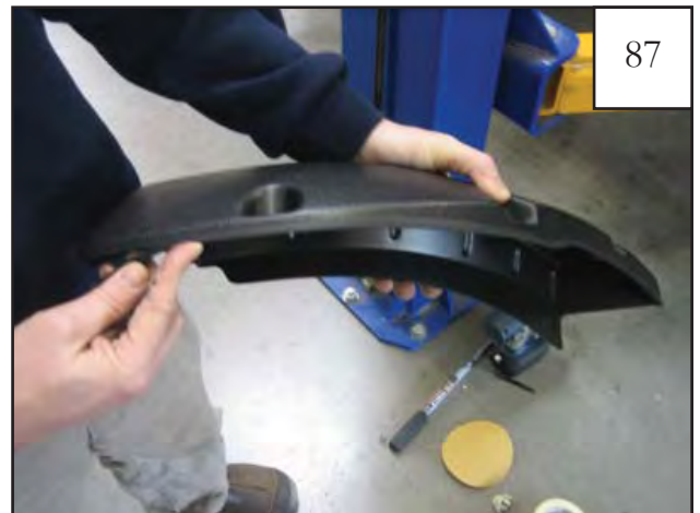
For edge trim application on rear door piece, follow steps as listed at the beginning of this instruction set. Apply edge trim only to the outer edge of the door piece.
