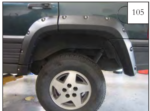
Completed rear flare installation.
