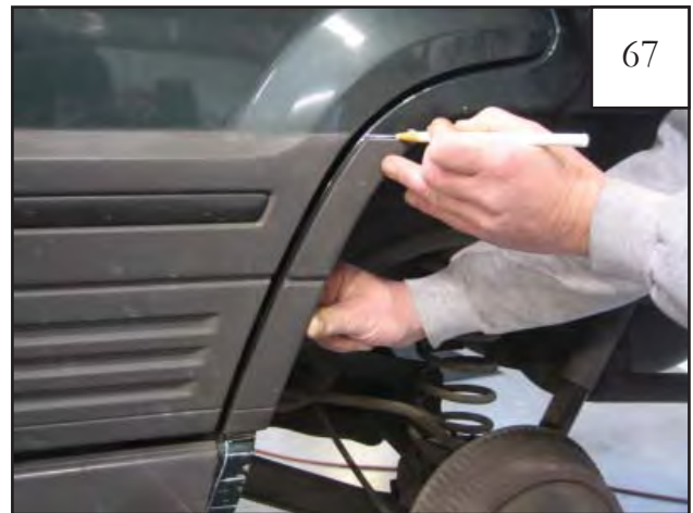
Hold factory side cladding to "dog leg" are of wheel well and trace a line at the top of the cladding on the vehicle.
