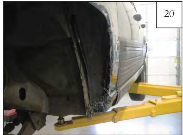
Using a heavy hammer, pound bent tabs securely into place over splash shield.
