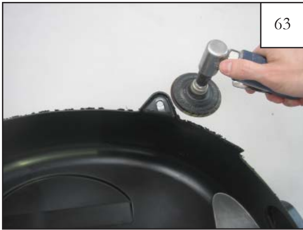
Sand mounting tabs flat using an angle grinder or sand paper.
